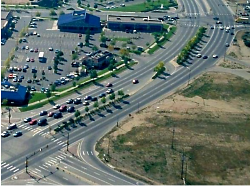
Figure 10. The photograph shows a raised median that restricts left-turn egress movements from a driveway located between two signalized intersections.
