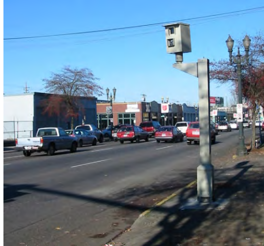
Figure 3. Enforcement cameras, as shown in the photo above, are used at signalized intersections to identify red light runners.
